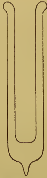
FIG. 9.—Double-walled glass vessels—so-called vacuum vessels. Owing to the absence of air between the walls, hot liquids put in such vessels remain hot, cold liquids remain cold, for a remarkably long time.
